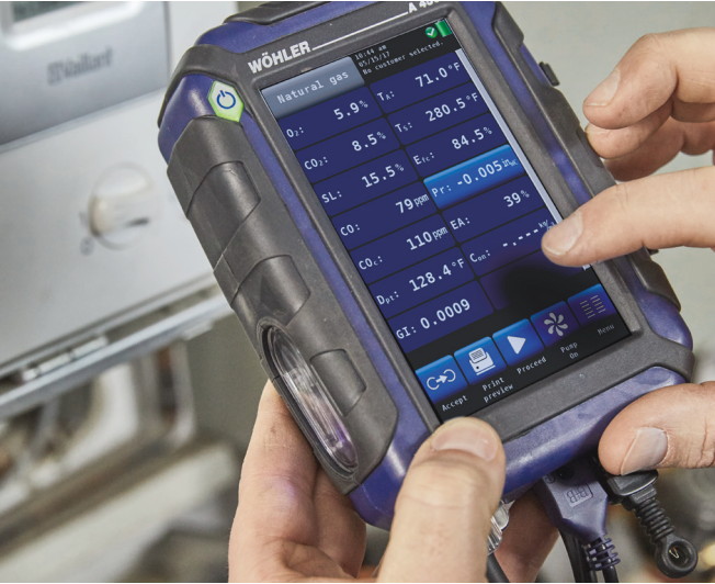
All measured values available at a glance thanks to high-resolution display
