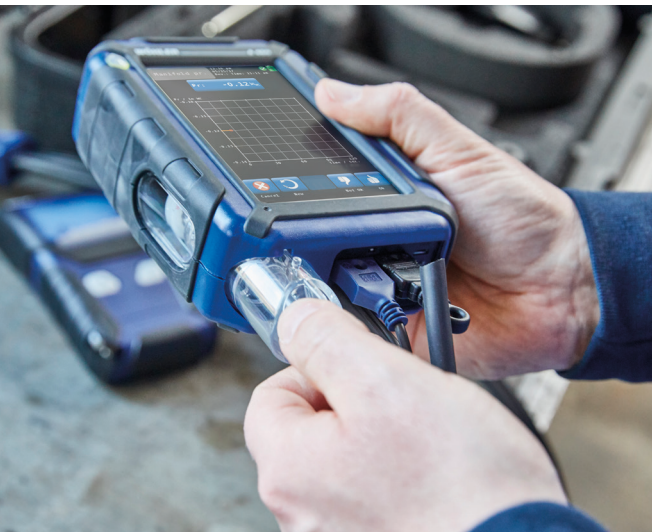
Simple maintenance – The condensate trap can easily be removed
